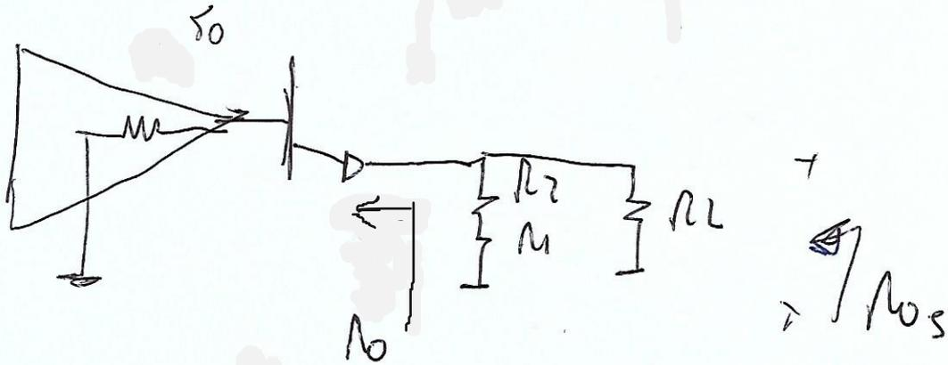
$$R_o = h_{ib} + \frac{r_o}{1+h_{fe}}$$
