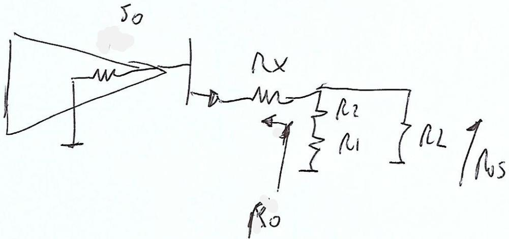
$$R_o = R_x + h_{ib} + \frac{r_o}{1+h_{fe}} \quad \text{with } R_x = 0,47 \Omega$$
