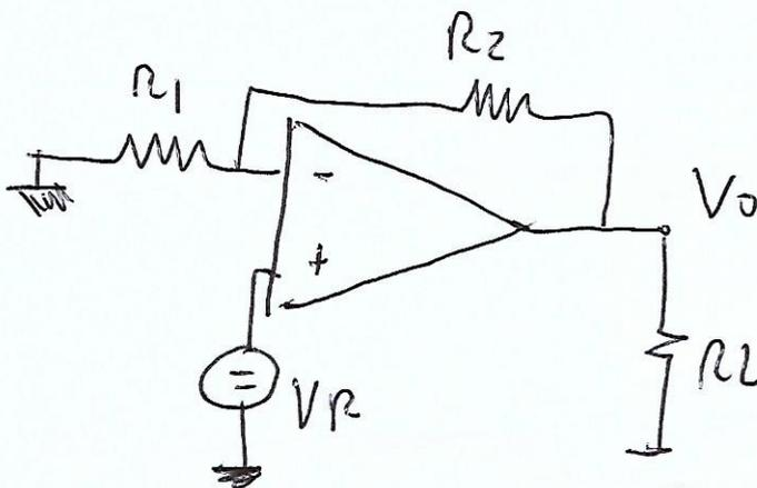
$$V_o = V_R \left( 1 + \frac{R_2}{R_1} \right)$$
