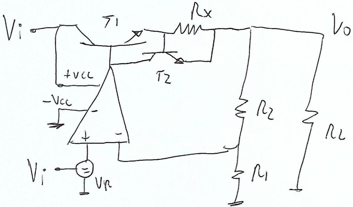
$$V_o = V_r \left( 1 + \frac{R_2}{R_1} \right)$$
