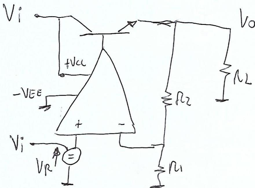
$$V_o = V_r \left( 1 + \frac{R_2}{R_1} \right)$$
