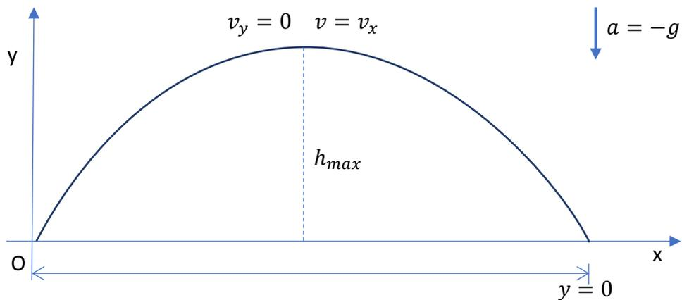
$$v_{0y} - g \cdot t = 0 \quad \Rightarrow \quad t = \frac{v_0 \cdot \text{sen}\alpha}{g}$$
