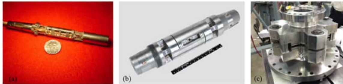
Figure 1: Internal and Semi-Span Strain Gage Balance Examples: (a) Small 20 lb. Normal Force Internal Balance used in 31-Inch Mach 10 Wind Tunnel (LaRC) (b) Large 5000 lb Normal Force Internal Balance used in 14 x 22 ft Subsonic Wind Tunnel (LaRC) (c) Large 30000 lb Normal Force Semi-span Balance used at 11 ft Transonic Tunnel (ARC).
