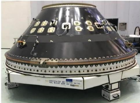
Figure 3-1: SpaceX 1,575-mm payload attach fitting
