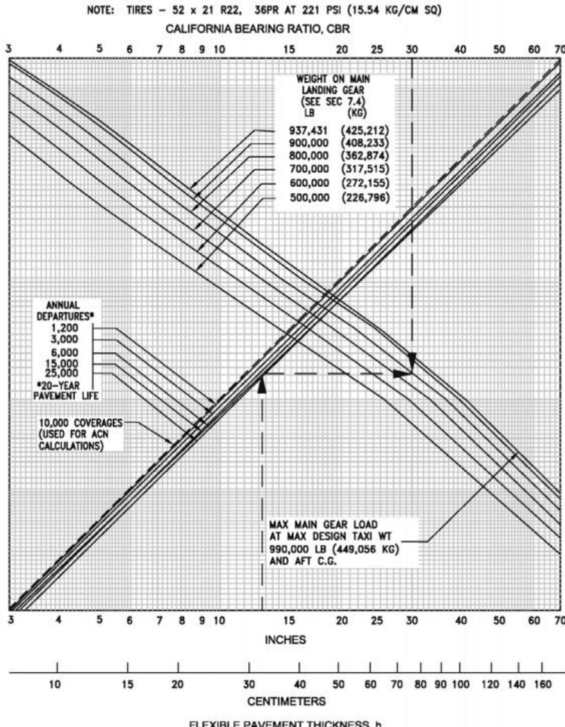
**7.5.2 FLEXIBLE PAVEMENT REQUIREMENTS - U.S. ARMY CORPS OF ENGINEERS
