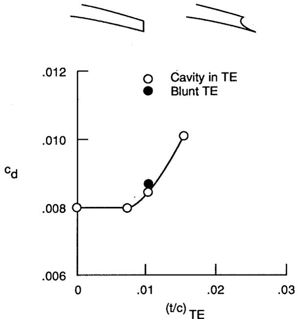
Figure 12. Effect of trailing-edge thickness on subcritical drag coefficient for 10-percent-thick refined supercritical airfoil.  $M = 0.60$ ,  $c_n = 0.60$ .
