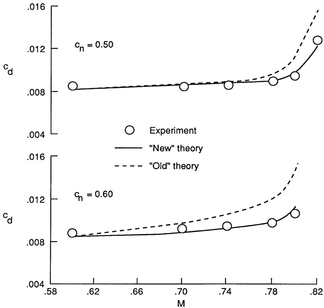
Figure 16. Comparison of experimental and analytical drag characteristics for supercritical airfoil 27.
