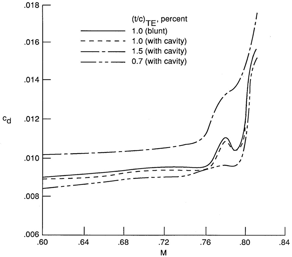
Figure 11. Effect of trailing-edge geometry on variation of section drag coefficient with Mach number at a normal-force coefficient of 0.7 for the 10-percent-thick refined supercritical airfoil.
