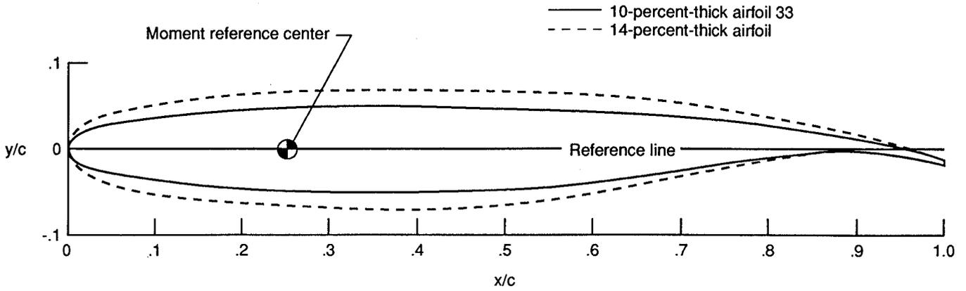
Figure 19. Comparison of 14-percent-thick airfoil with 10-percent-thick airfoil 33.
