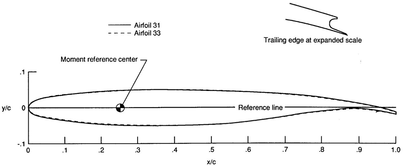
Figure 20. Sketches of 10-percent-thick supercritical airfoils 31 and 33.
