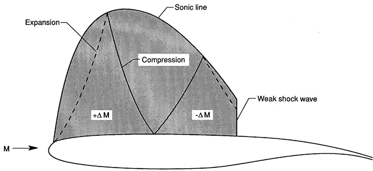
Figure 6. Schematic flow field of supercritical airfoil.
