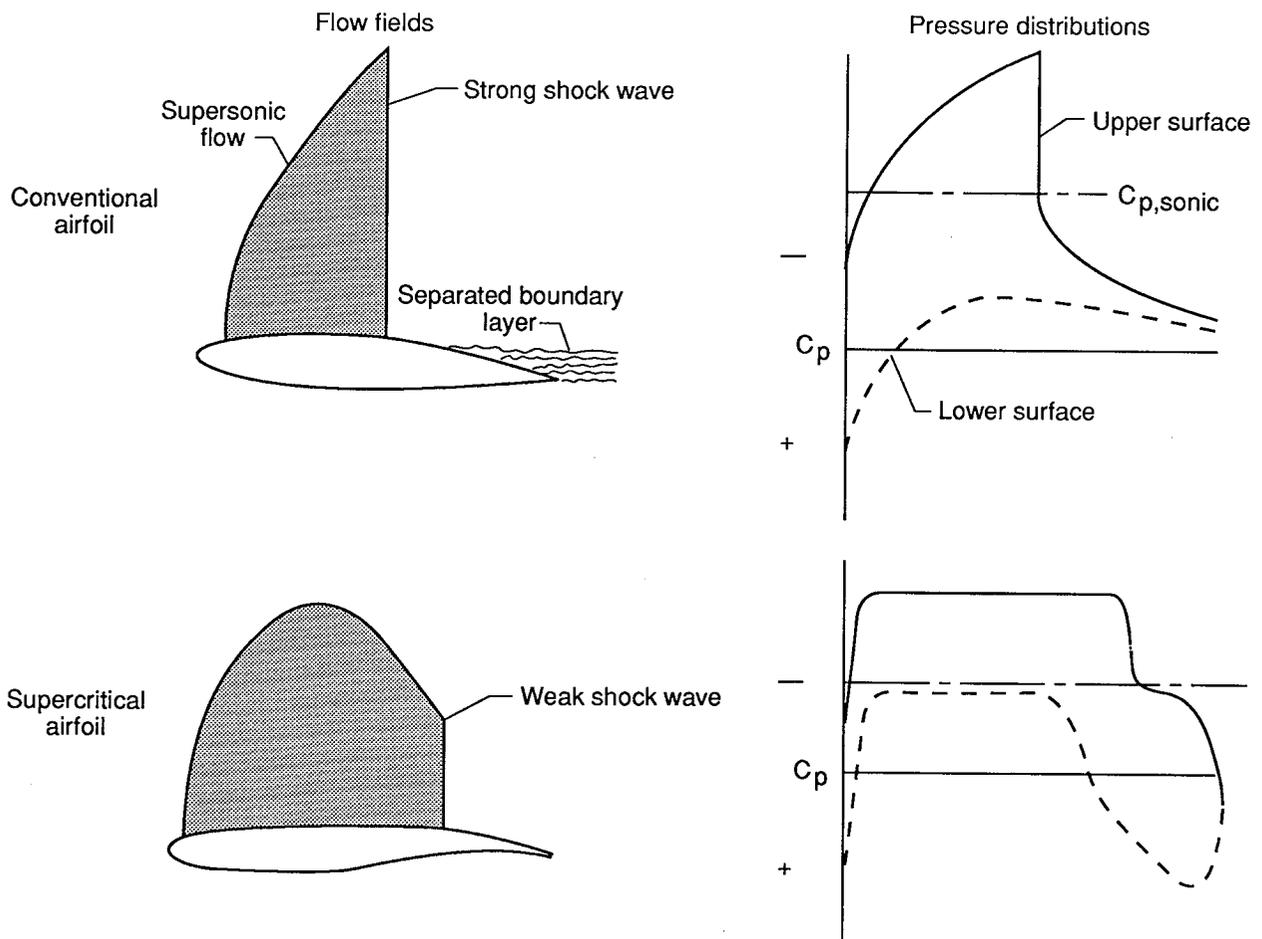
Figure 5. Flow fields around supercritical and conventional airfoils.
