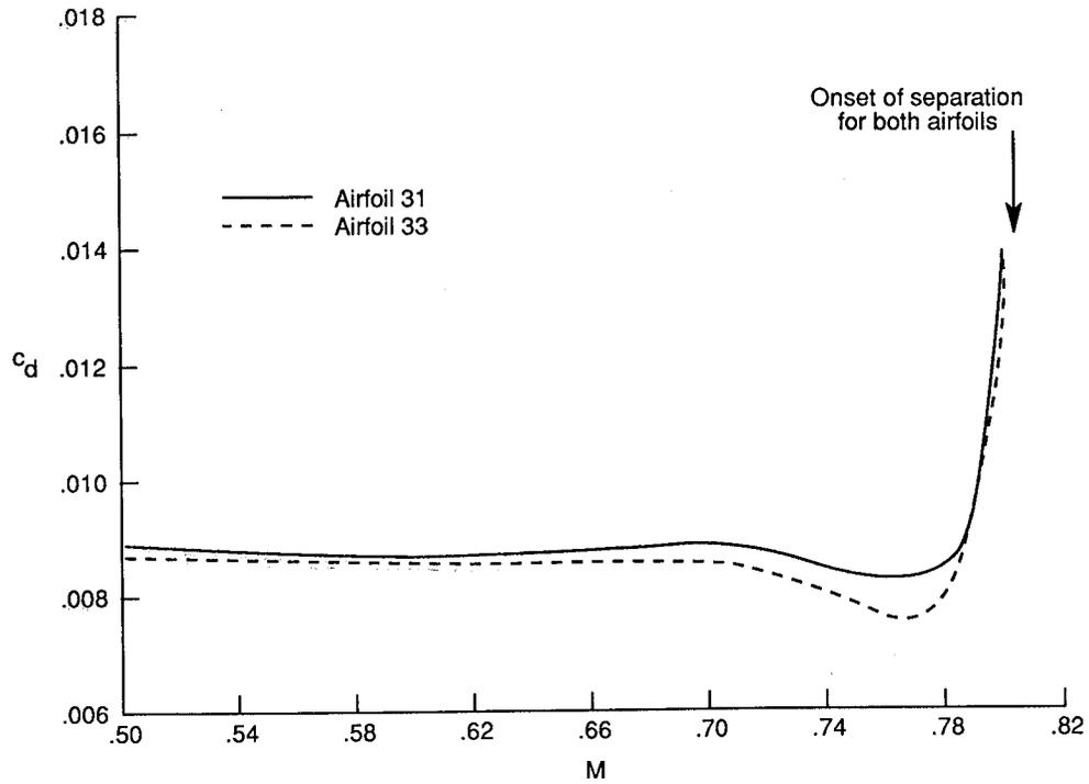
Figure 23. Experimental drag characteristics for supercritical airfoils 31 and 33.
