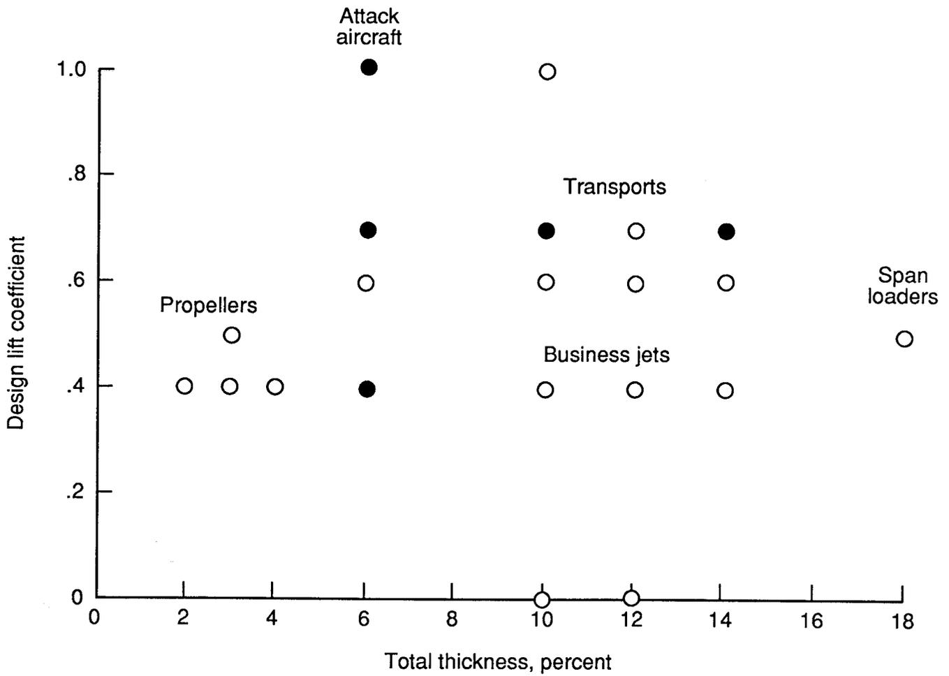
Figure 25. Matrix of phase 2 supercritical airfoils.
