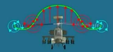
THE AUTOROTATIVE STATE IS THE BOUNDARY BETWEEN CONDITIONS WHERE ENGINE POWER MUST BE DELIVERED TO THE ROTOR TO PREVENT ROTOR RPM DECAY AND WHERE POWER MUST BE EXTRACTED FROM THE ROTOR SYSTEM TO PREVENT ROTOR OVERSPEED.
