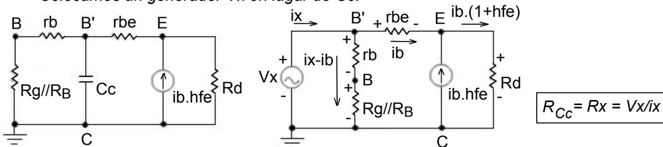
$$V_x = (i_x - i_b) \cdot (r_b + R_g // R_B) = i_b \cdot (r_{be} + R_d \cdot (1 + h_{fe}))$$
