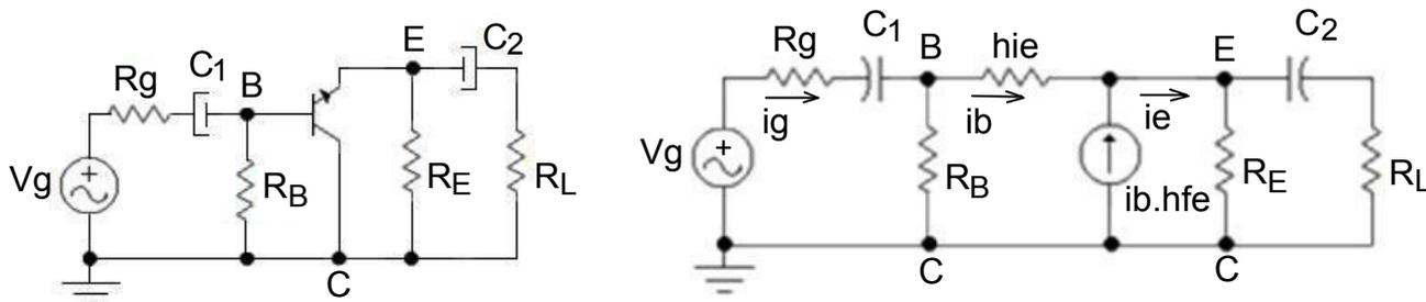
$$\tau_1 = C_1 \cdot R_1 = C_1 \cdot R_{is} = C_1 \cdot (R_g + R_B // R_i)$$
